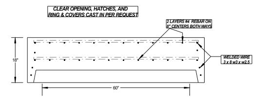
MEETS OR EXCEEDS ASTM C478 ---4000~# REINFORCED CONCRETE IN 28 DAYS
